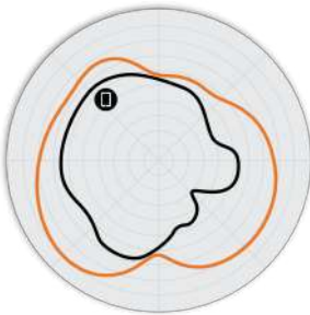
Figure 2. R350 2.4GHz Azimuth Antenna Patterns
