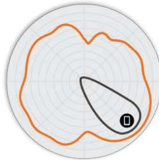
Figure 4. R550 2.4GHz Elevation Antenna Patterns
