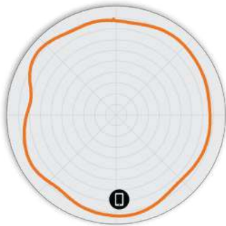
Figure 2. R550 2.4GHz Azimuth Antenna Patterns
